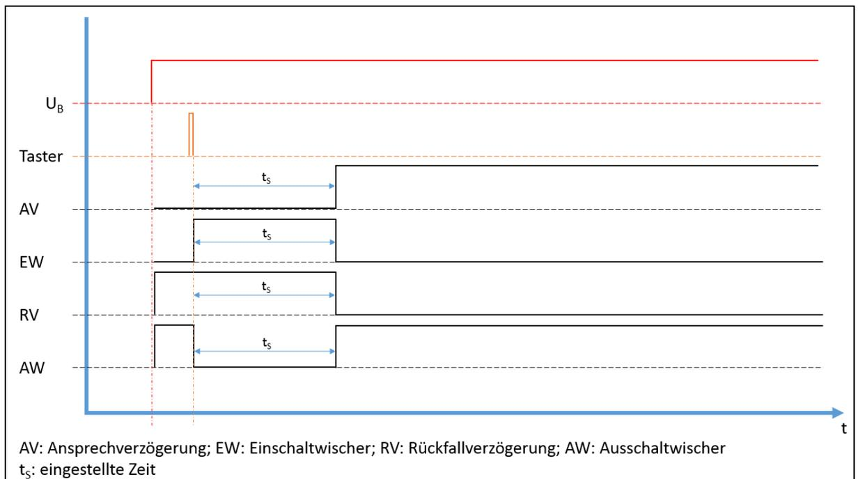
Figure 7: Overview of unlocked time functions
