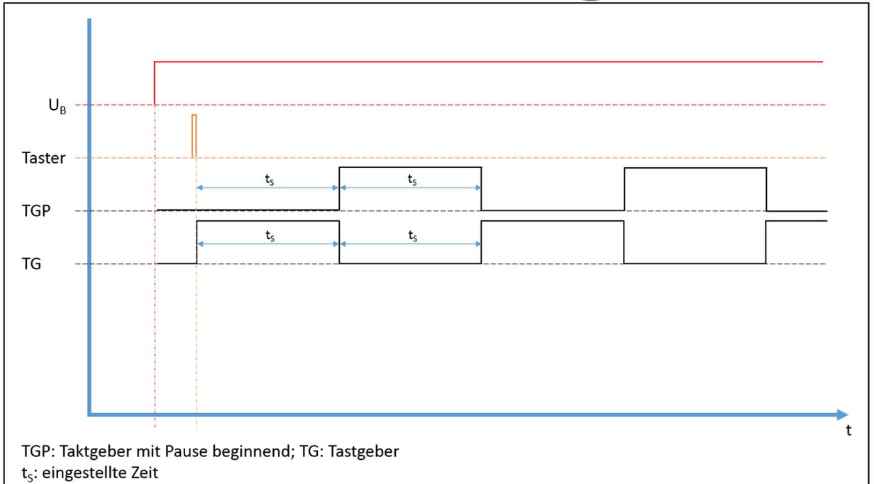
Figure 8: Overview of the clocked time functions
