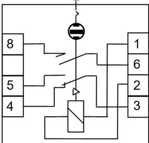
Version with 1 changeover contact and 1 passing contact
