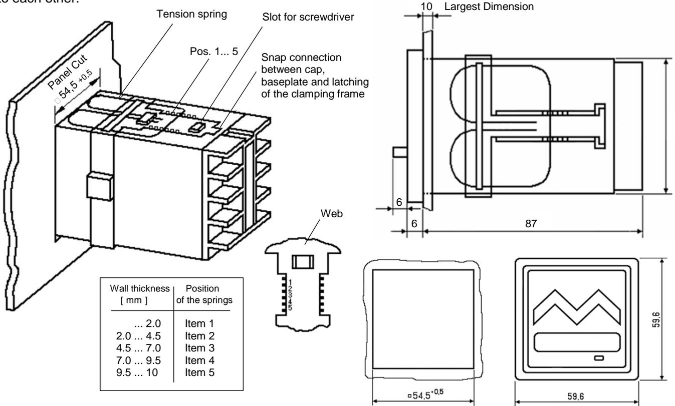
Clamping frame installation diagram
