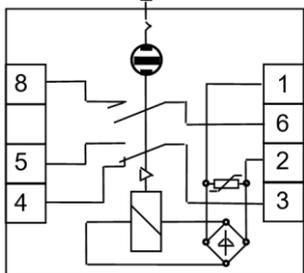
Version with 1 changeover contact and 1 passing contact
